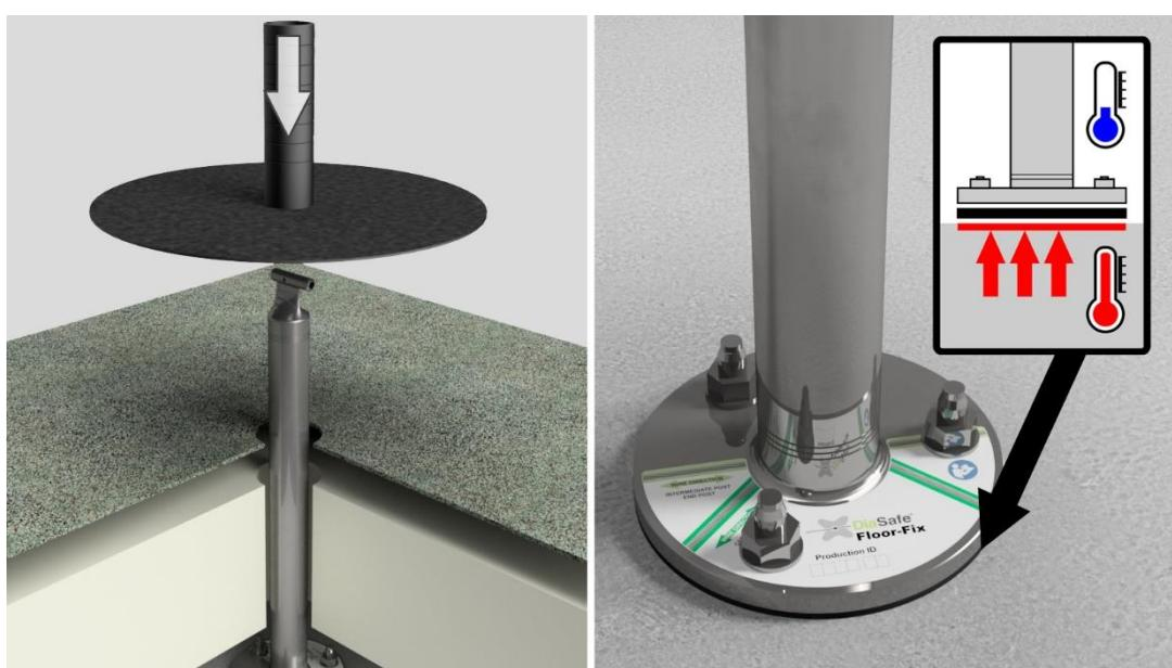
**Open linesystem installation (with start- and end posts) / Montageablauf
